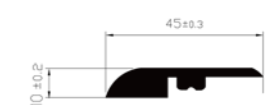
REDUCER To connect different level floors or floor end at threshold and to protect flooring
